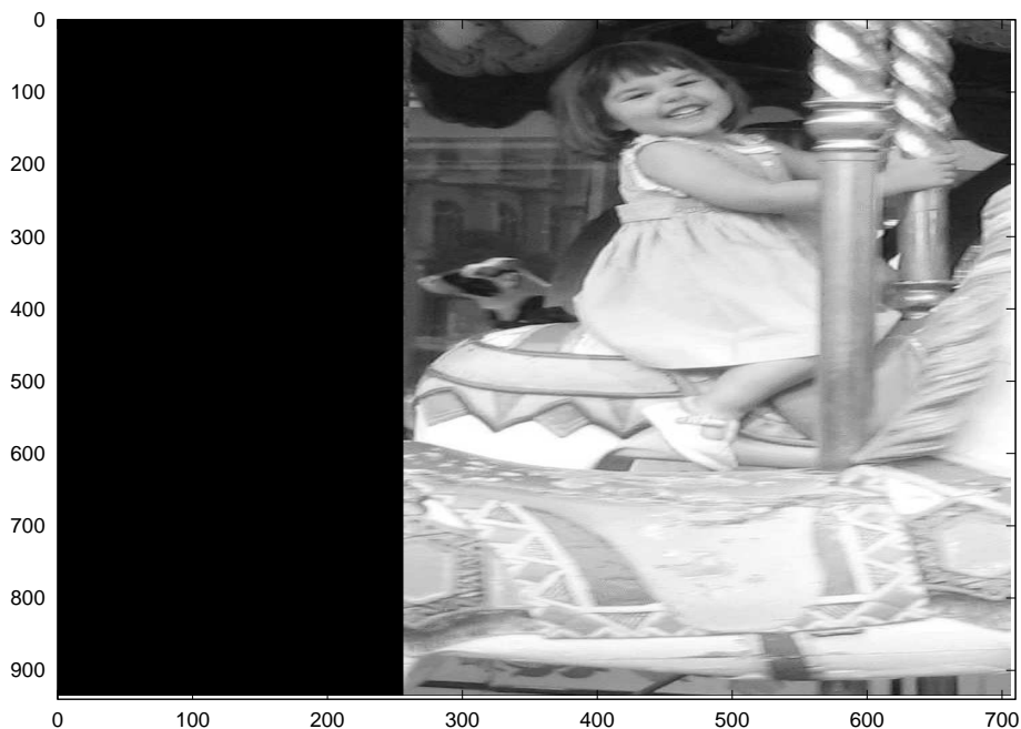
Figure 5.18: The result of convolving the photo in Figure 5.17 with a two-dimensional shift kernel. The kernel shifts the image 256 pixels in x and 0 pixels in y.
