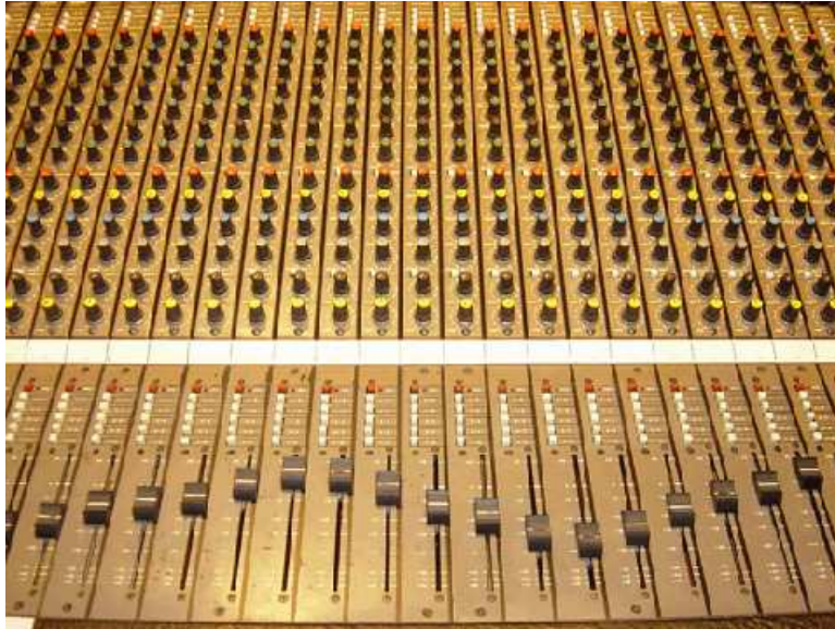
Figure 5.1: A contemporary mixing console features long-throw faders for attenuating an input signal and a set of equalizers (EQ) for altering the relative balance of the frequency content of each channel's audio signal. The input channels are routed to the output, typically stereo, via an audio buss.
