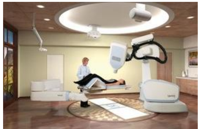
Figure 2. Illustration of the CyberKnife treatment setting’s main components, on the left side the RoboCouch with a patient, on the right side the radiation source mounted on a robotic arm. (Copyright: Accuray Inc.).
