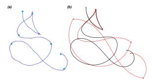
**Figure 7:** Fitting a  $\Gamma \Lambda \star$  trajectory to a sketched letter S. (a) A shaky input trace (magenta), the smoothed input trace (dashed turquoise) and the corresponding dominant points (turquoise circles). (b) The reconstructed trajectory and the corresponding action plan (red).
