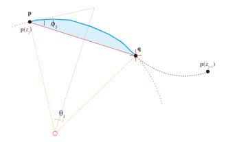
**Figure 8:** Computing  $\phi_1$  by fitting a circular arc between the first point of the contour section  $p(z_j)$  and the inflection at q.  $\phi_2$  will be computed similarly between the inflection (red cross) and  $p(z_{i+1})$ .
