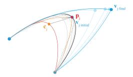
Figure 10: Iterative fitting: The initial action plan (orange) generates a trajectory (red) that is scaled with respect to the original (dashed grey). Through successive iterations the initial virtual target position moves until the corresponding point along the trajectory (orange circle) converges towards the input segmentation point (red circle).
