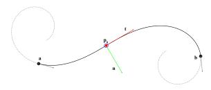
**Figure 5:** Definition of an Euler spiral connecting two Hermite points **a** and **b** based on Walton and Meek's definition.
