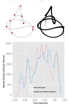
**Figure 12:** Fitting a  $\Gamma\Lambda^*$  trajectory. Top Left: the input contour and corresponding segmentation points. Top Right: the generated trajectory. Bottom: The velocity of the generated trajectory (red) overlapped with a manually scaled and aligned version of the input velocity signal (turquoise).
